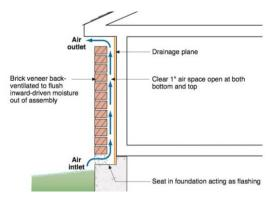
Figure 3: Back ventilation for brick veneer walls.
